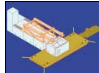
Lift-in Construction Method for Lock Wall Construction.
