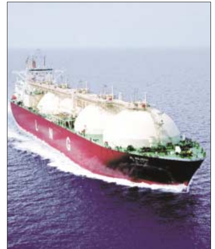
Example of a 137,000 m 3 Liquefied gas carrier.
