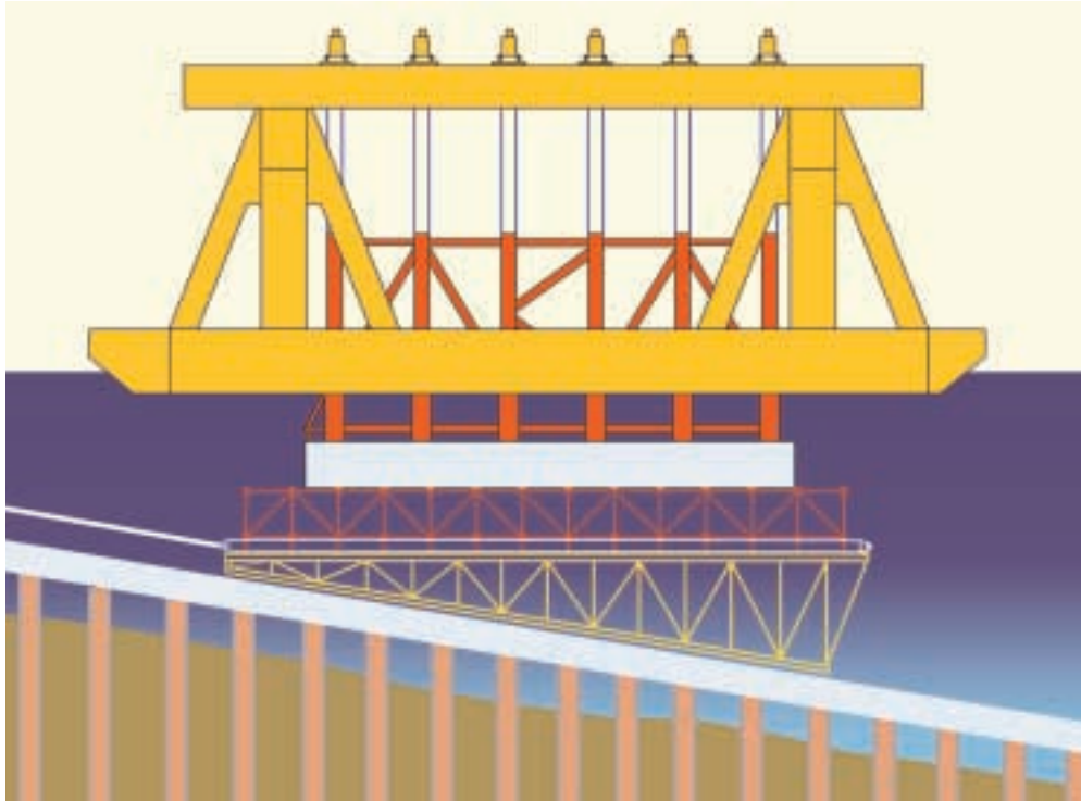
Catamaran Preparing to Lift the Frame and Shell Off of the Sled for Transport to its Final Location
