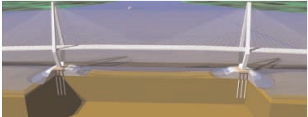
Rendering of the New Cooper River Bridge and Artificial Pier Protection Islands
