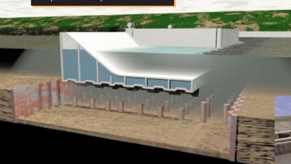
Dam positioned over pre-installed caissons
