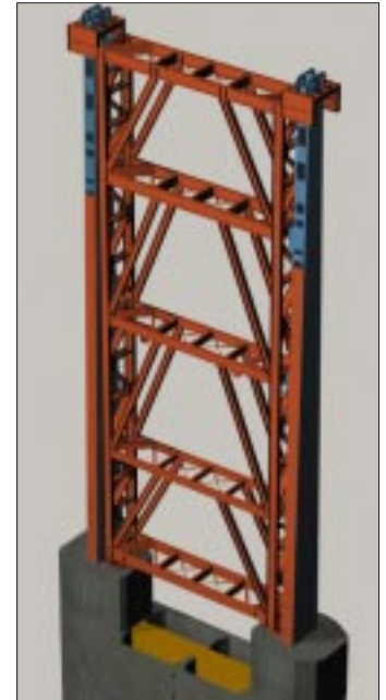
Dual EBF tower retrofit.
