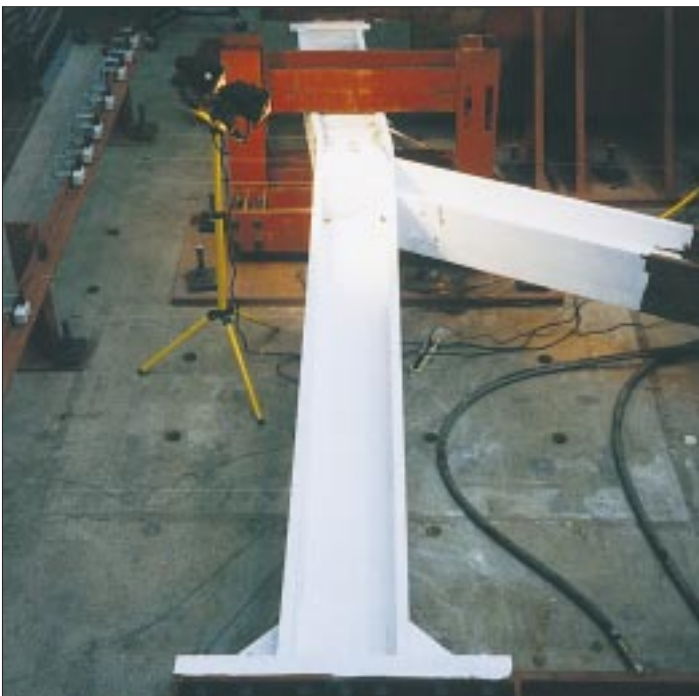
Test specimen - built-up beam and diagonal.
