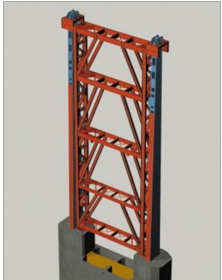
Dual EBF tower retrofit.
