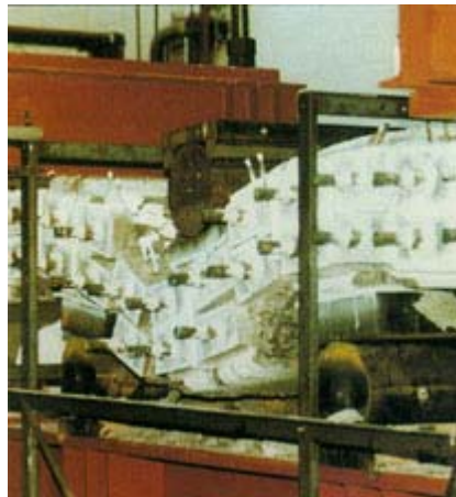
Test specimen with 100% of ultimate capacity and a deflection ductility factor of over 40
