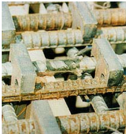
T-Heads of Stirrups used in Testing Program
