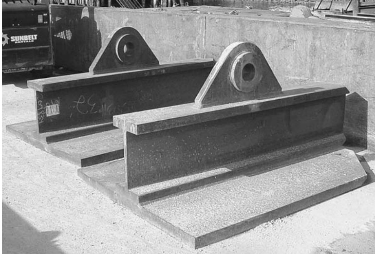
FIG. 1 Driven plate anchor
