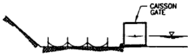
① CONSTRUCT BASE CAISSON IN CONSTRUCTION BASIN
