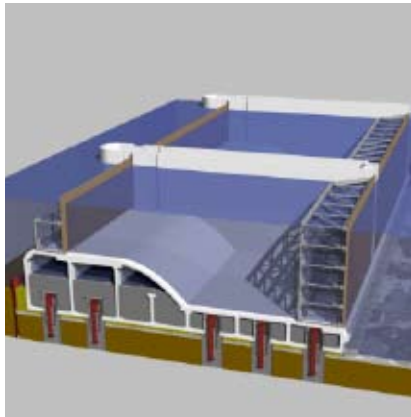
In-the-wet dam construction - tremie infill of dam segment positioned over pre-installed caissons.
